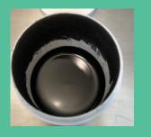
Flowing slurry at >80 % solid = less NMP
